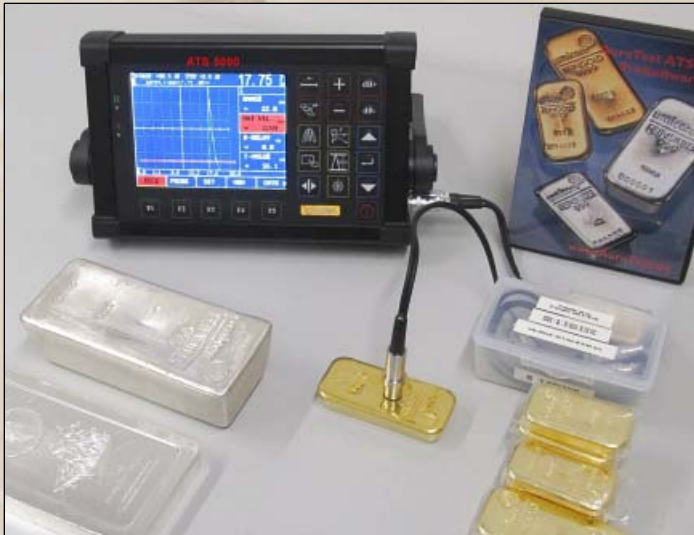
ATS 5000 with intermediate size sound probe attached to a 1 kg Umicore gold bar; other bars up to 5 kg silver or 100 oz in preparation for testing
